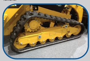
To prepare the track for the backside of its lifespan, steel cords and inserts are dipped to allow strong adhesive bonding while encasing the internal track with preventative corrosive coats. The factory does not produce generic guides nor molds; each track is designed specifically for the application and model intended.
